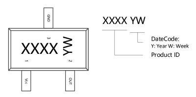
Figure.13 SOT-23 Chip Marking Spec
