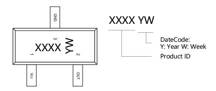
Figure.15 SOT-23 (Thin Outline) Chip Marking Spec
