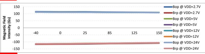
Figure.9 MT8962-Plus Magnetic Characteristics (Bop & Brp) vs. Vdd @ Temperature=25°C
