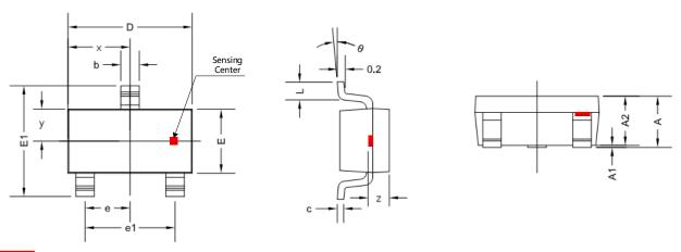
Figure.14 SOT-23 Package Drawing
