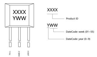
Figure.17 Flat TO-92 Chip Marking Spec
