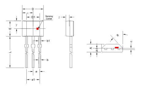
Figure.18 Flat TO-92 Package Drawing
